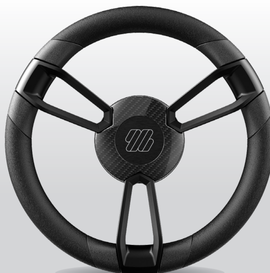
Manna PU B/B/CB 25897V Ø 350 mm (13.8") - Depth: 95 mm (3.74") Black polyurethane grip, black stainless steel spokes, carbon look cover
